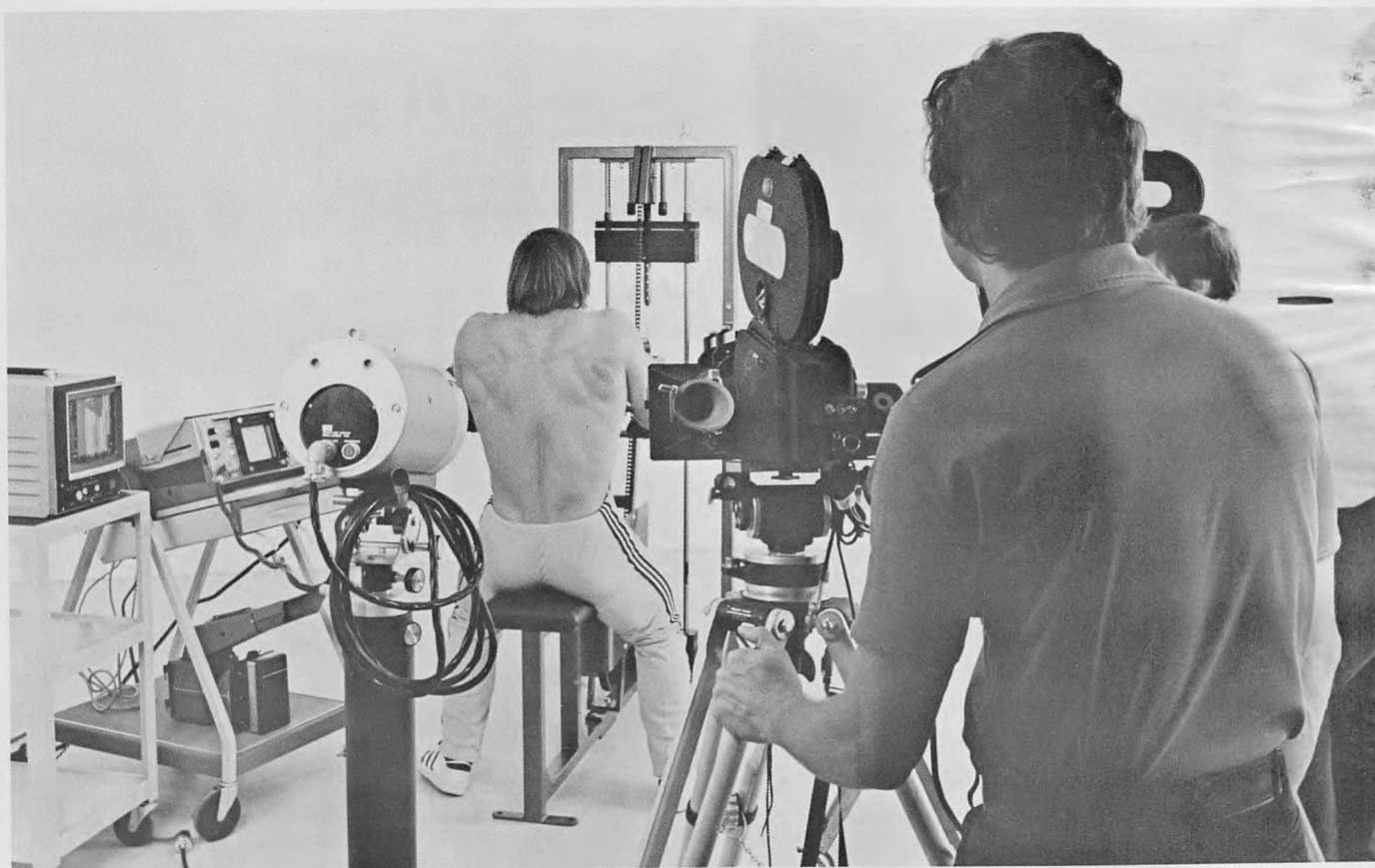
Electronic Scanning Infrared Camera focused on the upper back of a trainee using a Nautilus Neck and Shoulder Machine.
